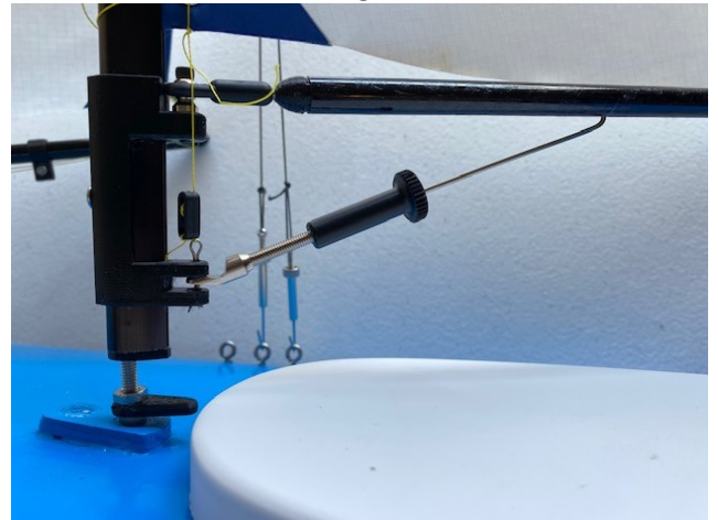
Details of Goose Neck, Boom Vang, and Downhaul
