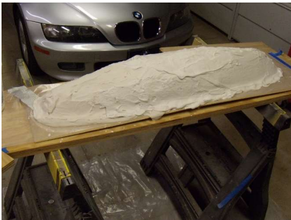
Casting the hull mold
