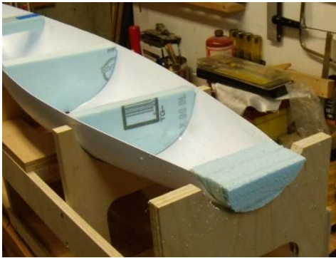
Modifying the Soling hull transom prior to casting the mold
