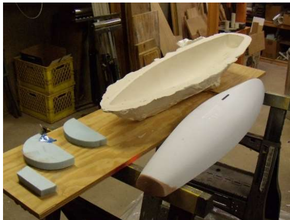
Hull mold with Soling hull removed
