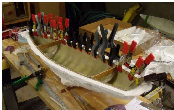
Glassing in the bulkheads and flanges
