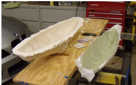
The first fiberglass hull removed from the mold
