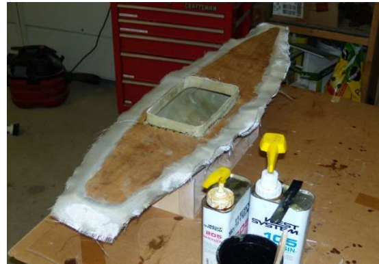
Deck and hatch glassed onto the hull
